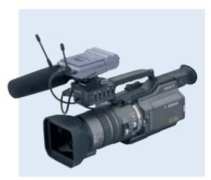
Photo shows portable tuner mounted on a camera.
